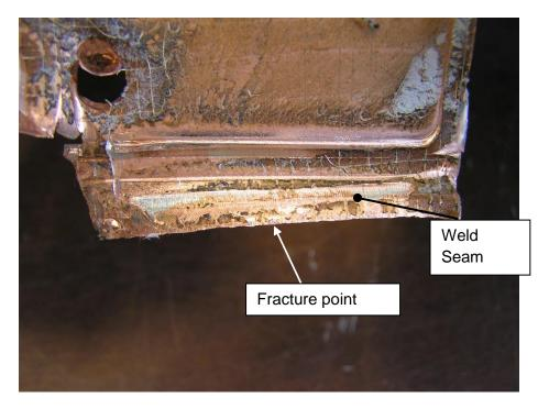
Figure 21 Fracture down one side of longitudinal weld seam (Image No. P1012790.jpg)
