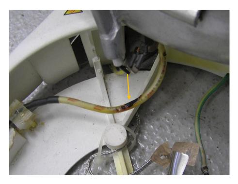
Figure 67 Heat damage to electrical fitting (arrow) in plastic base of autoclave 14426 (Image No. P1013001.jpg)
