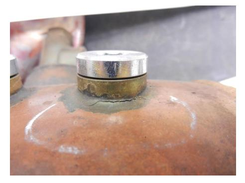
Figure 42 Crack through brazed joint in port fitting (Image No. DSCN5938.jpg)
