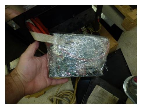
Figure 57Control PCB wrapped in Clingfilm (Image No. P1050959.jpg)None of the new café boilers had any such defects.
