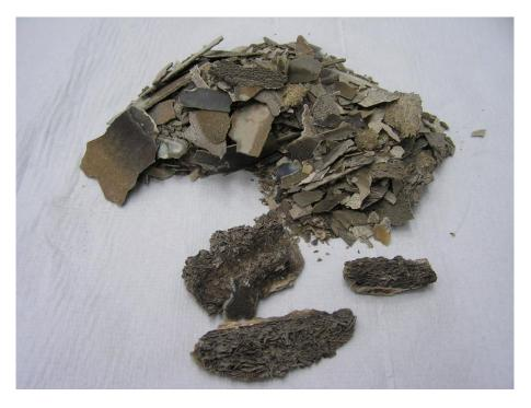
Figure 15 Lime-scale accumulated in base of vessel (Image No. P1012978.jpg)
