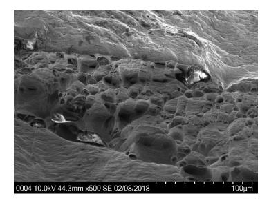
Figure 24 Higher magnification electron micrograph showing ductile microvoid coalescence at failure point. (Image No. 14373 fract\_0004.jpg)
