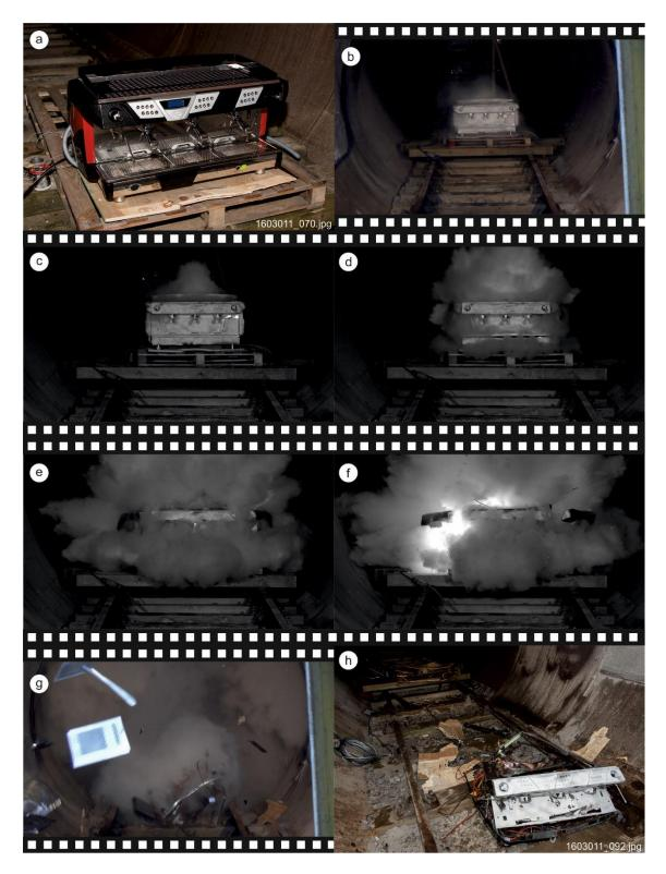
Figure 19 Images from the test – manufacturer A (new)
