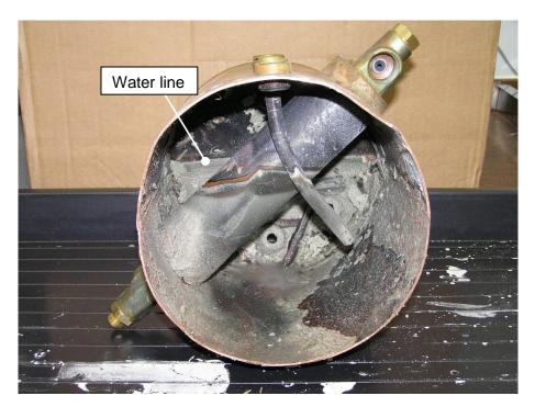
Figure 9 Interior of vessel showing lime-scale deposits (Image No. P1010867.jpg)
