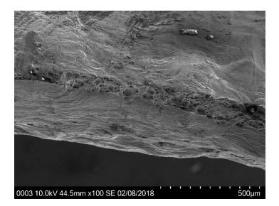
Figure 23 Electron micrograph – looking edge-on to the fracture. (Image No. 14373 fract\_0003.jpg)
