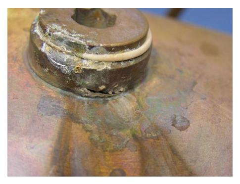
Figure 50 Cracking in wall of fitting at drain port (Image No. P1012939.jpg)
