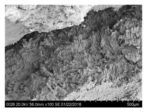
Figure 51 Fracture surface of the crack (Image No. 14430\_0026.jpg)
