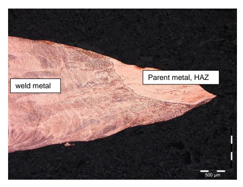
Figure 22 Tapered ductile fracture point of vessel, adjacent to weld. (Image No. 14373 met-1-1.jpg)
