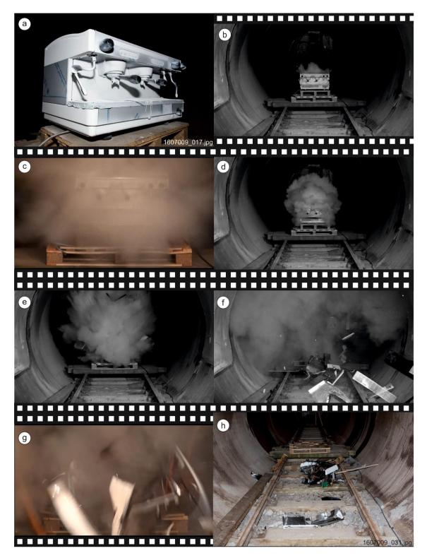
Figure 33 Images from the test – manufacturer D (new)
