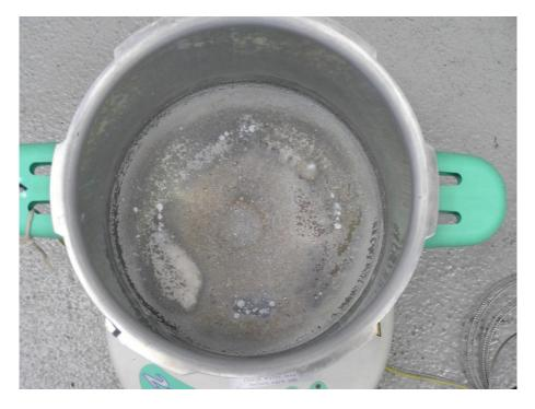
Figure 65 Base of 2nd hand autoclave 14426 after overpressure testing (Image No. P1012998.jpg)
