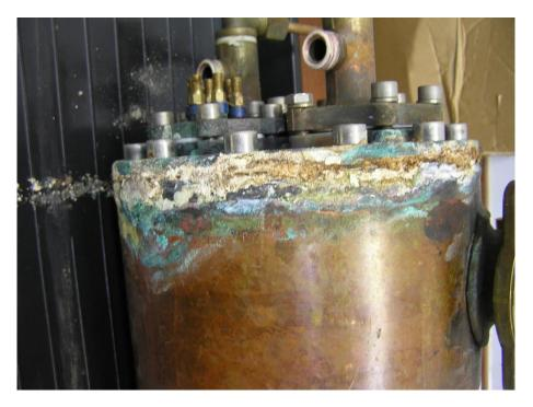
Figure 5 Corrosion deposits at end plate (Image No. P2202727.jpg)
