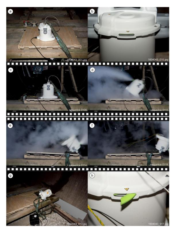
Figure 59 Overpressure testing of new autoclave 14427
