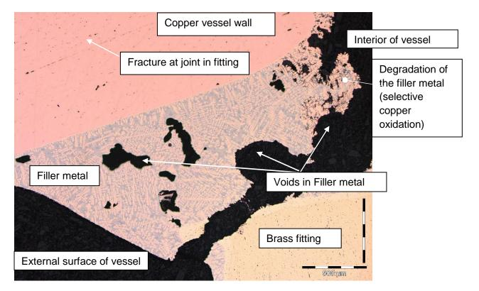
Figure 39 Cross section through cracked brazed joint (inset shows fractured joint at low magnification) (Image No. 14035 met1-1.jpg)
