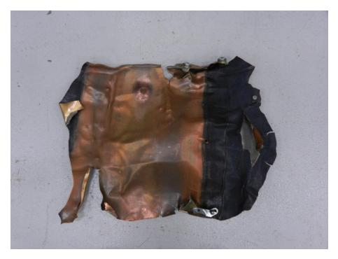
Figure 47 Section of fractured boiler vessel (Image No. DSCN5957.jpg)
