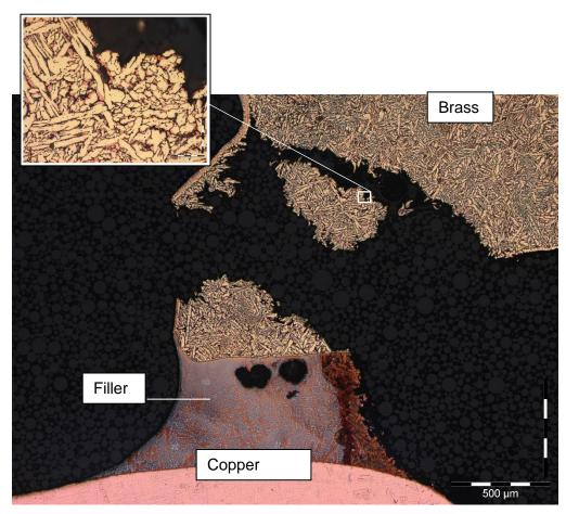
Figure 52 Cross-section through fractured drain port fitting (inset showing pink copper-rich regions due to zinc depletion (dezincification)) (Images No. 14430 met 2-1a, 14430 met 2-5.jpg)
