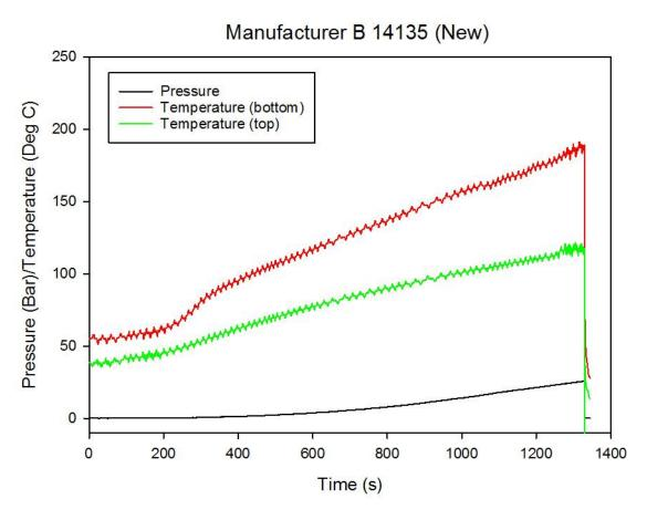
Figure 25 Pressure and Temperature Results – manufacturer B (new)
