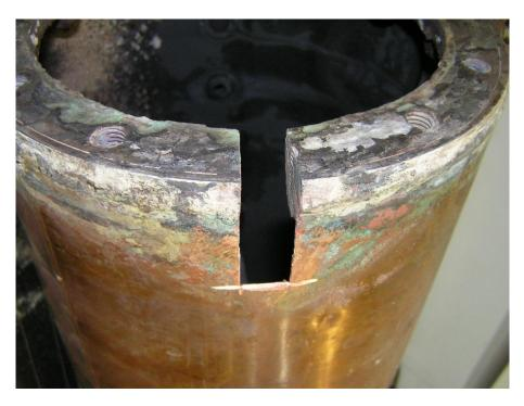
Figure 7 Section taken through the end plate weld (Image No. P1010834.jpg)
