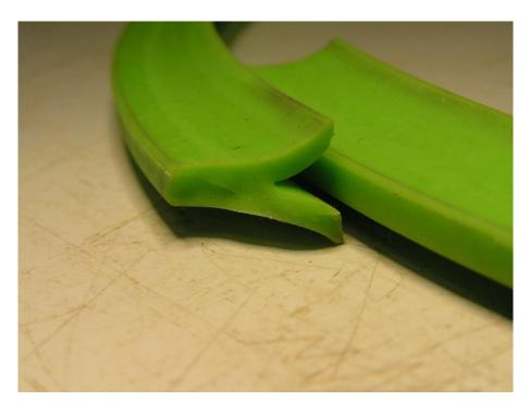
Figure 62 Ruptured gasket from autoclave 14427 (Image No. P1012991.jpg)
