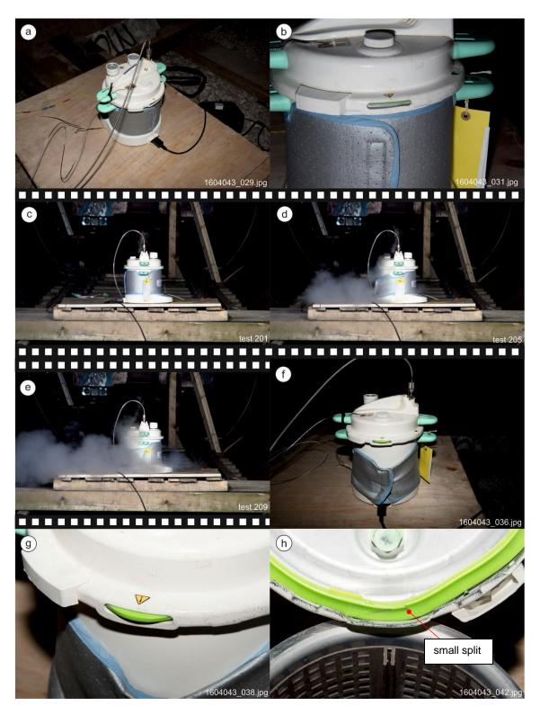
Figure 61 Overpressure testing of 2nd hand autoclave 14426
