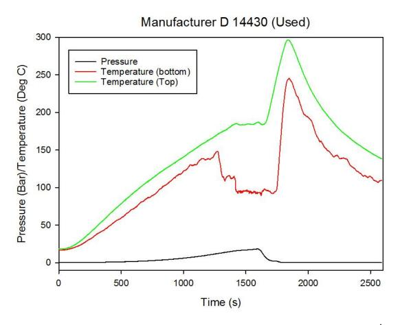
Figure 48 Pressure and Temperature Results – manufacturer D – 2<sup>nd</sup> hand (used)
