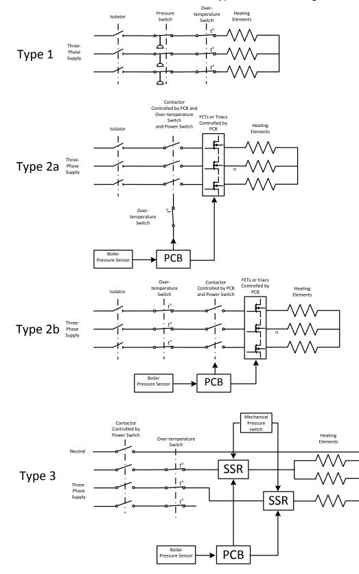
A schematic of the electrical control circuit types is shown in Figure 2.
