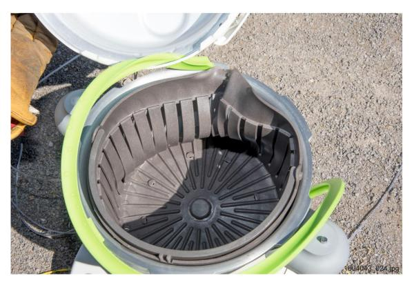
Figure 60 Deformation of internal carrier basket, new autoclave 14427 (Image No. AIS 1604043\_024)
