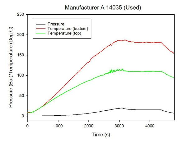
Figure 35 Pressure and Temperature Results – manufacturer A –2nd hand (used)
