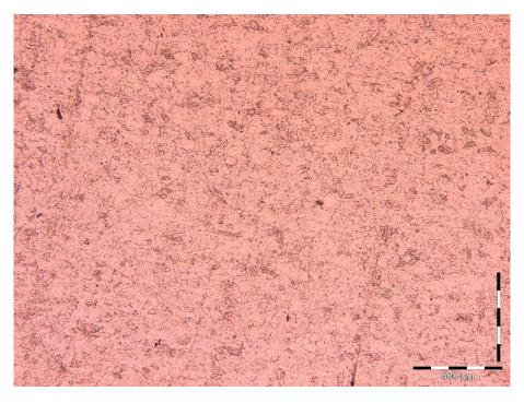
Figure 10 Fine equiaxed grain structure in parent strip (Image No. 14134 met1-3.jpg)
