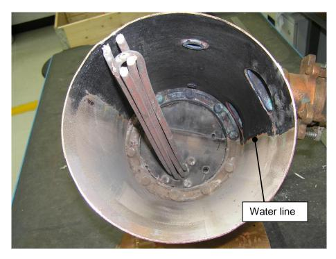
Figure 13 Interior of boiler vessel (Image No. P1012987.jpg)
