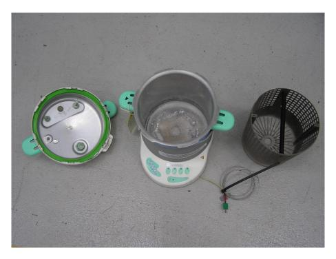
Figure 64 Components of 2nd hand autoclave 14426 after overpressure testing (Image No. P1013005.jpg)
