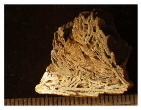
Figure 16 Solid deposit of lime-scale from vicinity of heating element (divisions on scale are millimetres) (Image No. 14432 massive scale.jpg)
