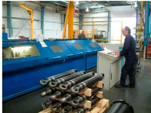
Figure 3 An enclosure for hydraulic cylinders fitted with access panels that are locked in place during a test to prevent access. Visual examination for leaks is done through a polycarbonate section in the panels
